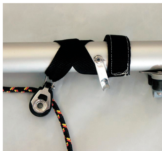
Strapping the forward block to the boom.
