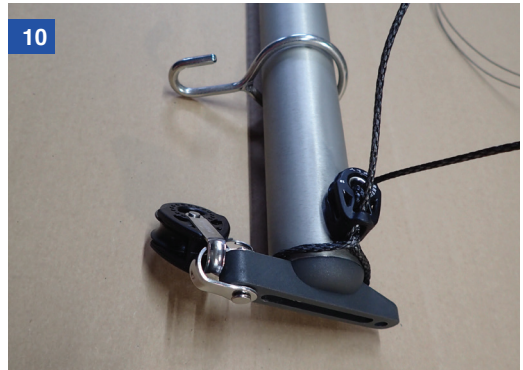
Pull the other dyneema tail through the hole in the top of the pulley and out the opposite side to the other tail, meaning that they are now both on the same side of the pulley
