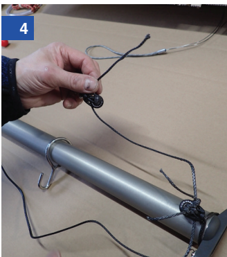
Then pass the end through the new pulley with the karabiner attached
