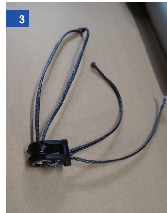
Using the fid, thread the middle part of the dyneema down through the hole in the top of the pulley, out to one side and then through the centre of the pulley
