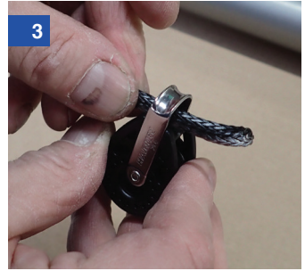
Double up the dyneema and put the middle part through the metal loop on the pulley
