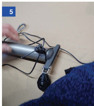
Finally, thread the end through the outside upper hole in the boom end fitting
