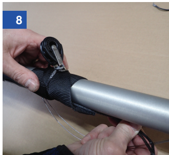
Repeat for the other end of the dyneema, the other side of the rivetted washer which is on the upper side of the boom
