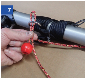
Make a loop in the rope near the bobble and feed it through the metal kicking strap ring attached to the webbing
