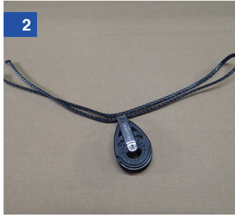
For this you need the mainsheet pulley and 30cm (11.8in) length of dyneema
