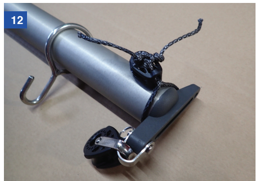
Finishing off with an overhand knot on each dyneema tail, with the knot as close to the reef knot as possible
