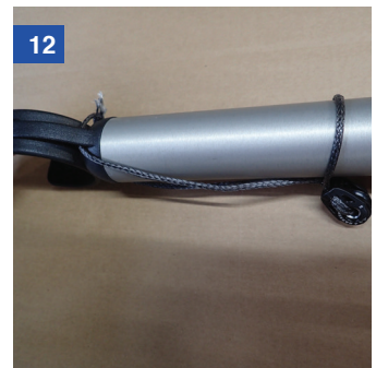
Pull the pulley along the boom away from the gooseneck – it should be 10cm (4in) from the gooseneck
