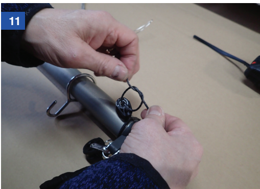
Now tie both dyneema ends together with a reef knot
