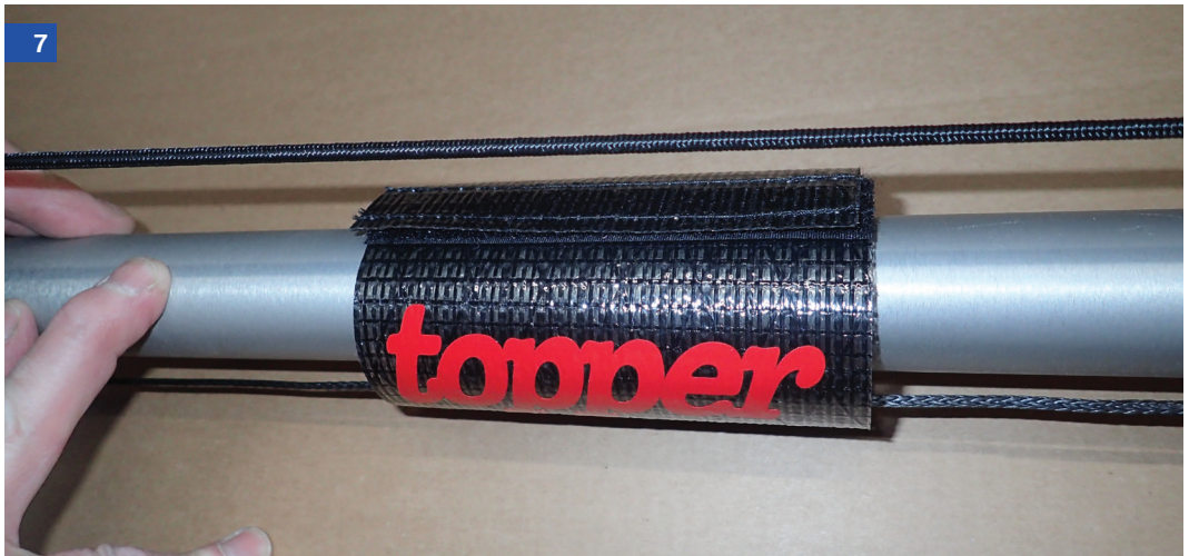
The grey outhaul line (below the boom) passes through the mylar strap, but the black outhaul shockcord does not
