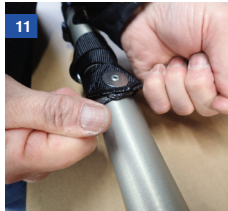
Making sure that the knot is tight against the rivetted washer under the strapping
