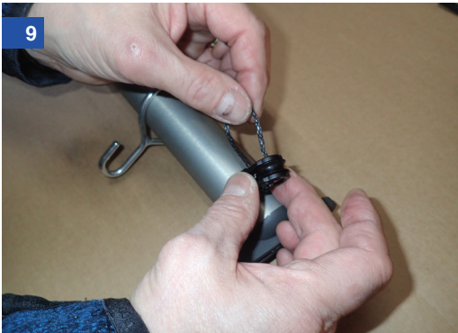
Then thread the same tail through the hole in the centre of the pulley
