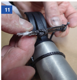
And then tie each in another overhand knot over the other end of dyneema and pull tight
