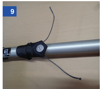
Pull tight so the pulley is held tight against the webbing strap and is on the underside of the boom (the same side as the outhaul cleat)
