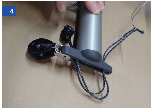
Now thread the tails through the inner upper hole in the boom end fitting
