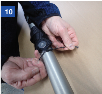
Tie the two ends of dyneema together with a reef knot
