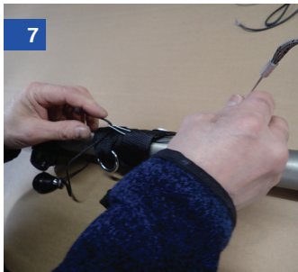
Using the fid, pull one end of the dyneema through the webbing strap
