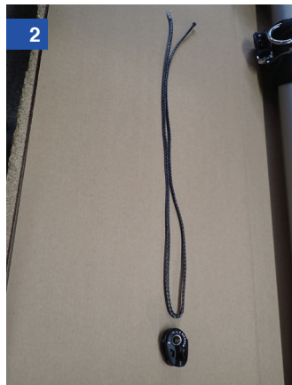
For this you will need the outhaul pulley and 52cm (20.5in) length of dyneema, which you double up
