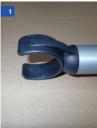
You will be attaching the forward outhaul pulley to the boom and the boom gooseneck fitting, which looks like this when supplied
