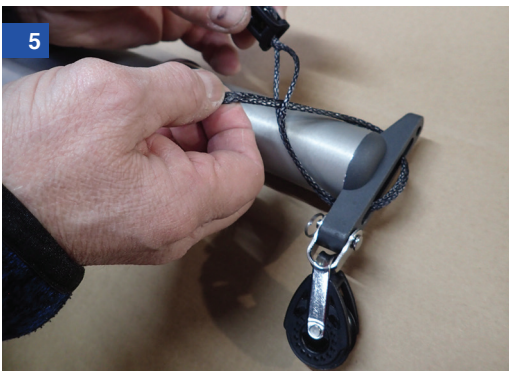
Pass the dyneema tails through the loop by the rear outhaul pulley
