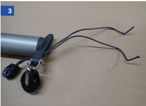
Using the fid, thread the dyneema tails through the inner bottom hole in the boom end fitting – next to where you have already attached the stern mainsheet pulley
