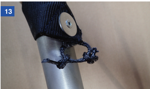
Then tie each in another overhand knot over the other end of dyneema
