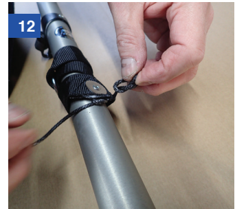
Tie an overhand knot at the end of each loose end of dyneema
