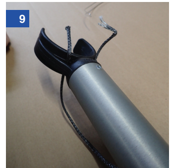
Thread these through the holes in the gooseneck, going from the underside of the boom to the topside
