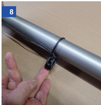
Using the fid, thread the loose ends of the dyneema through the loop around the boom
