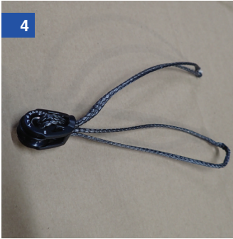
Then thread the middle part back up through the hole in the top of the pulley
