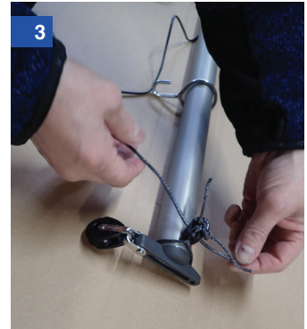
Pass it through the rear outhaul pulley you have just fitted
