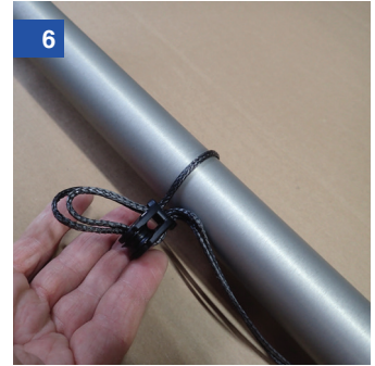
About 10cm (4in) from the end of the boom by the gooseneck, start tightening the loop round the boom by pulling through the dyneema to extend the loose ends
