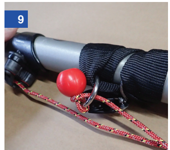
Then tighten to secure the end of the red line
