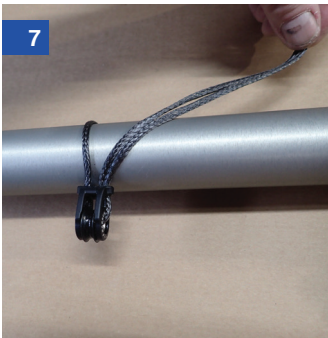
So the pulley is tight against the underside of the boom (same side as the outhaul cleat)
