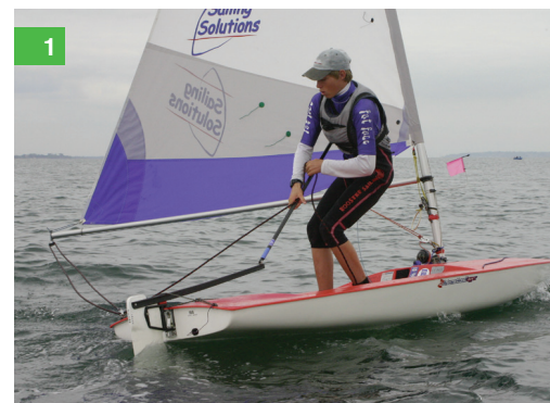
1 During the gybe, hold both the tiller extension and mainsheet with your old tiller hand (in this case, the right hand)
