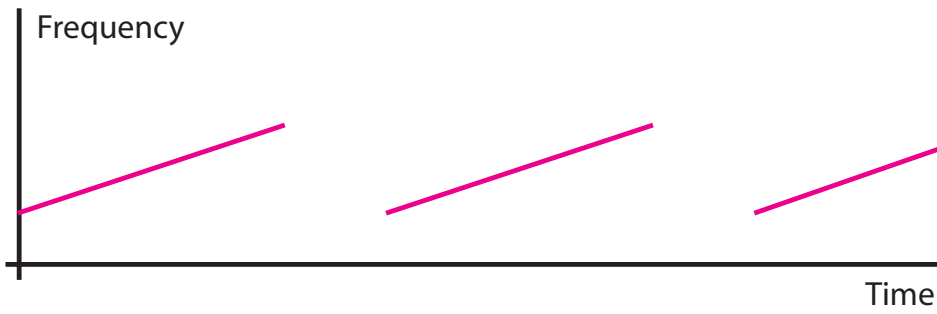
FIGURE 2 How FMCW radars calculate target range
